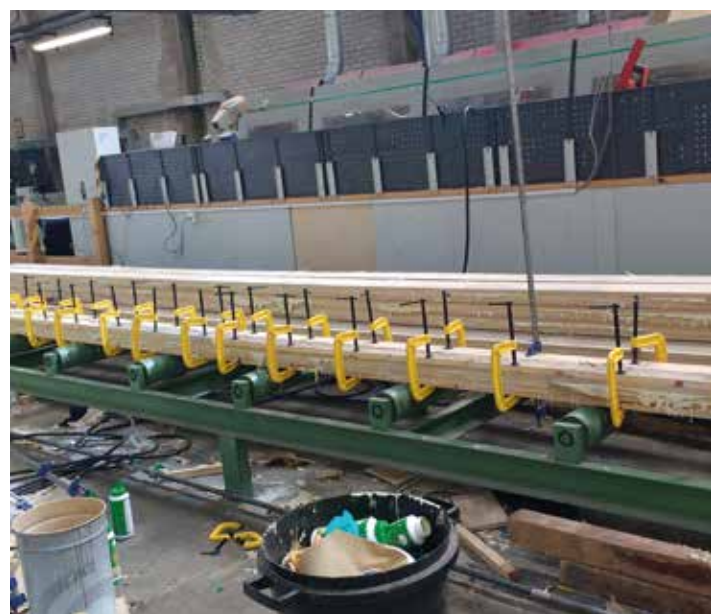
Example of a bespoke job using Accoya laminated using clamps
